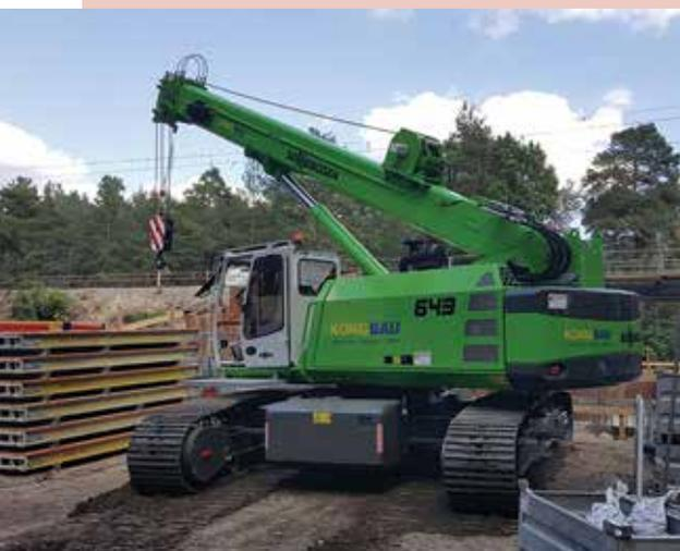
König Bau using a new Sennebogen 643 telescopic crane is used for a variety of lifting tasks.
